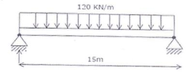
36:- The beam is subjected to a maximum bending moment of
